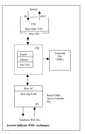
**Figure 1**. Block diagram illustrating the first tier components: Conversation I/O, Conversation Manager, and Application Code.
